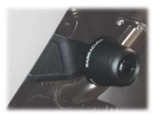
**LEFT SIDE:** attack point to the chassis. Use the thickness in kit
