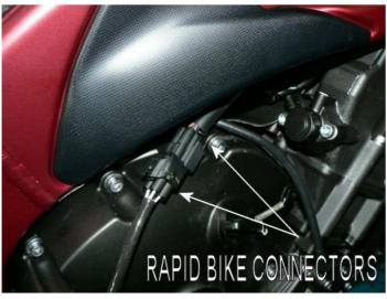
3. Connect the Rapid Bike connectors in-line with the stock ones.
