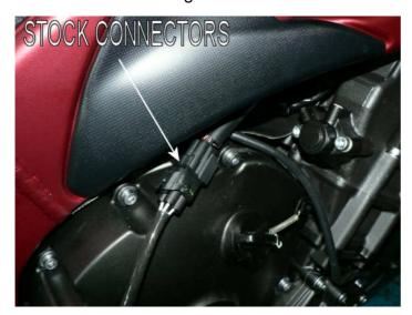
Locate and disconnect the 4 pin black connector of the o2 sensor.
