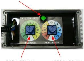
TRIMMER N°1 **TRIMMER N°2**  The green led shows the state of the device:
